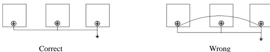
Figure 3-8 Grounding Wire Connection Sketch Map
